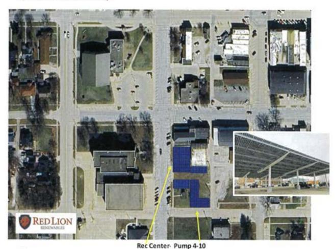
Jefferson combo\*\* S parking Solar Solar Array Size (kW-DC) 144 126 Solar Annual Production (kWh) 158,224 138,446 Current Annual Usage (kWh) 182,000 138,233 Electrical Usage Offset 86.9% 100.2%
