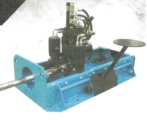
The Pit Shot is our latest direction drilling machine, designed with the utility contractor in mind. It has been engineered to operate soley as a pit launch machine, and exhibit up to 15,000 lbs. of push/pull force. The Pit Shot can install 1"- 6" pipes on grade, accurately up to 0.5%, making it ideal for sewer lines, water lines, and gas lines.
